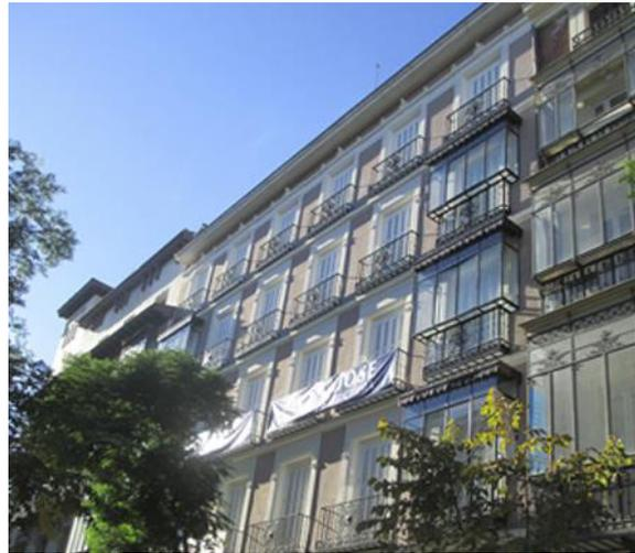
The building is located at N°6 in the Calle Salustiano de Olózaga in Madrid and dates back to the 19th Century and is a perfect example of the noble construction of this period: Load-bearing walls composed of a framework of studs and sleepers, braced with masonry brickwork and lime mortar. These walls were normally arranged parallel to the main façade, acted as supports to the wooden joist flooring which made up the five floors of the building.
